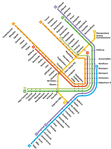
Fig. 6 S-bane line plan 2016 optimized with respect to minimizing the train driving minutes on lines running across two signalling systems.
