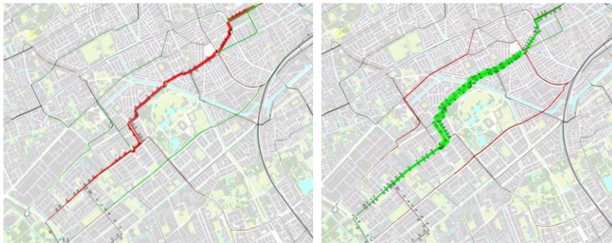
**Fig. 5:** Relative network effects of transformation of bus line 25 to tram line on link loads a) without considering comfort (left) and b) considering comfort effects (right) for a work day (excluding morning and evening peak).
