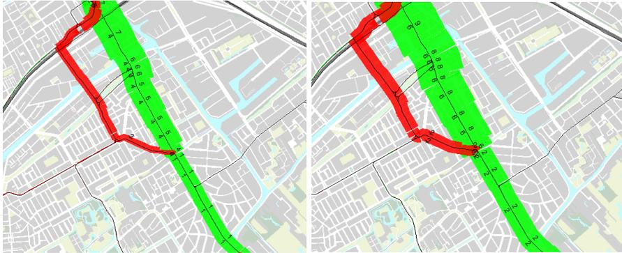
**Fig. 4:** Relative network effects of frequency increase on link loads a) without considering comfort (left) and b) considering comfort effects (right) during a morning peak.
