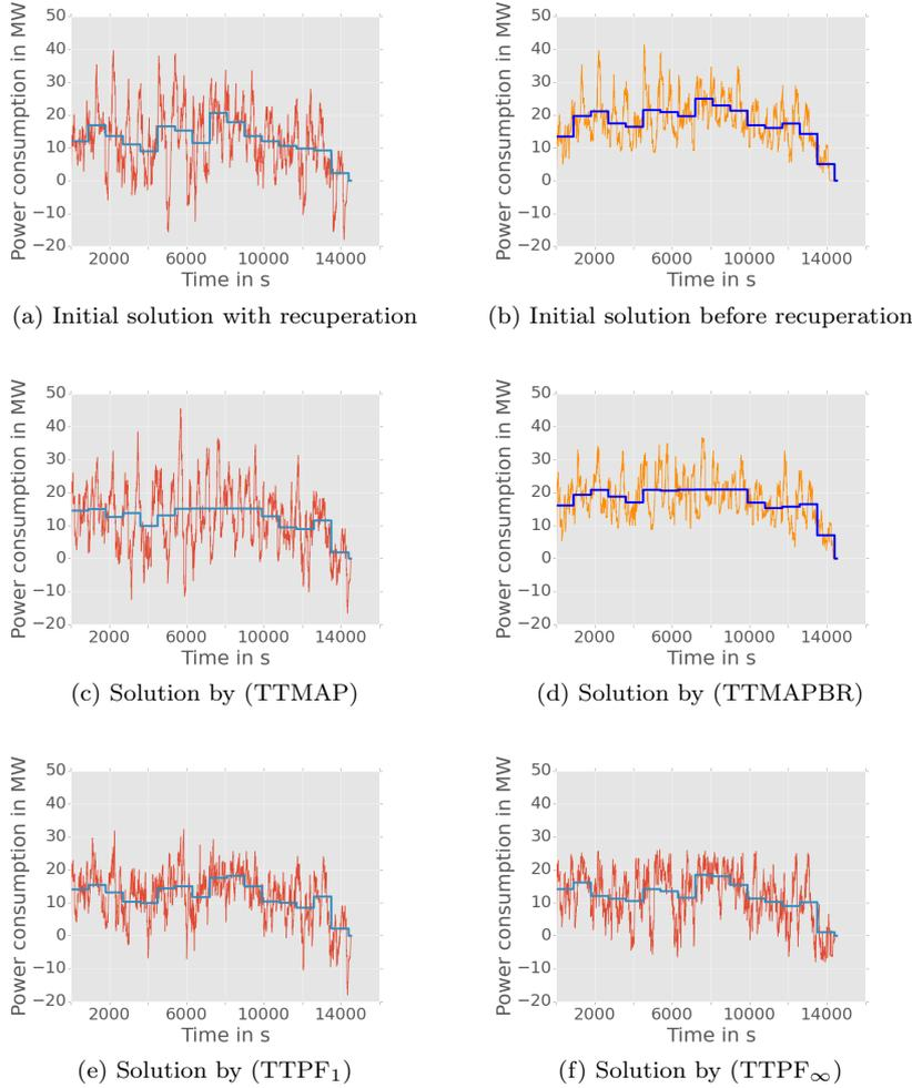
Fig. 3: Comparison of the system-wide power profile before and after optimization of test instance *Lichtenfels* under the different models considered here
