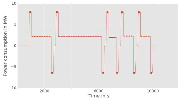
Fig. 2: The power profile of an ICE train on a journey with 5 trips
