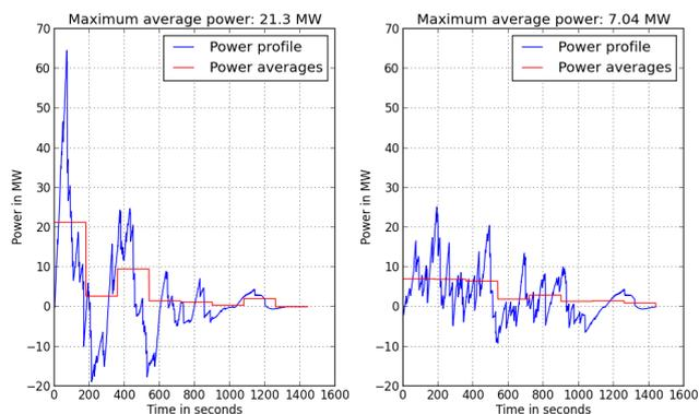
Fig. 1: Power load induced by railway traffic before (left) and after (right) optimization of the underlying timetable
